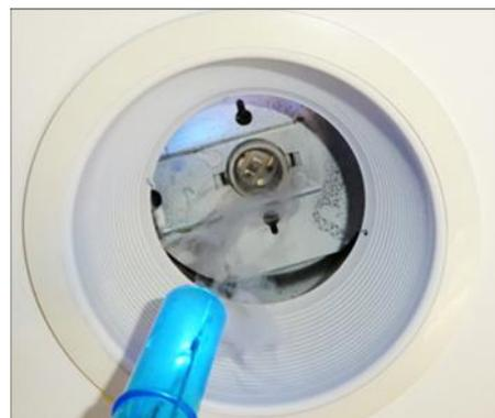
*Smoke pencil confirms airflow through a light fixture*
