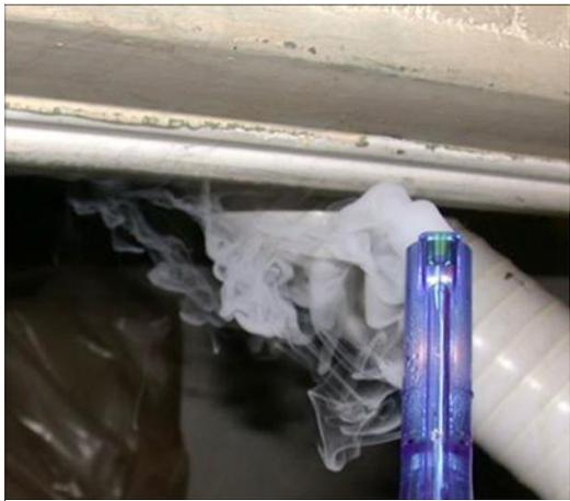
*A smoke pencil confirms warm air flow into a crawl space at the top of the basement-access window.*
