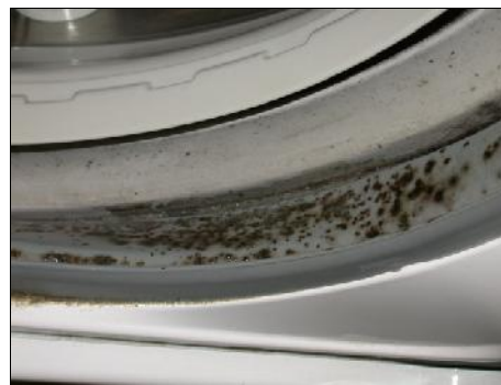
Washing machine with mold growth May Indoor Air Investigations LLC
